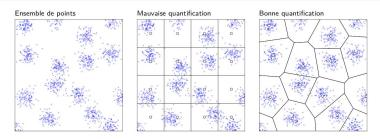
For 2D points, examples of a bad quantization and a good quantization
