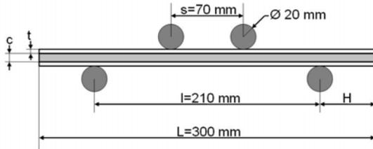
Fig. 2. Configuration of the four-points bending.
