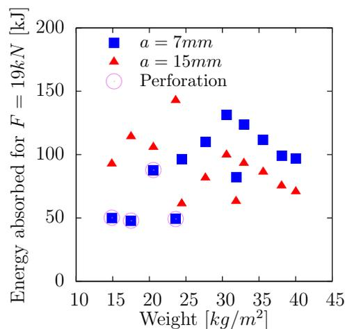
**Figure 3.14:** Energy absorbed for a load of 19kN among the surfacic weight of the structures. Energies for both indent sizes are presented. Marks of sandwich structures that failed by perforation are circled.
