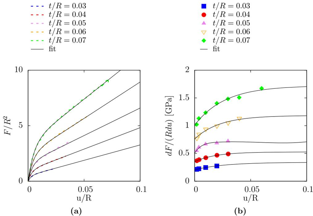
**Figure 2.10:** Simulations of 2 spheres without neck in compression. The shell thickness ( $t/R$ ) has been varied. Simulations and corresponding model for the stress-strain curve **(a)** and for the unloading modulus evolution with strain **(b)**.
