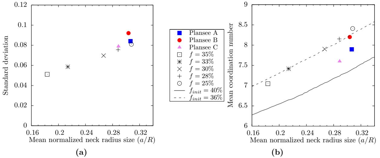
**Figure 2.14:** Comparison of the neck size scatter (a) and of the relation between the mean neck size and the mean coordination number (b), in the real and numerical samples. The mean coordination evolution with mean neck size is described both for samples of initial porosity  $f_{init}$  of 40% and 36%.
