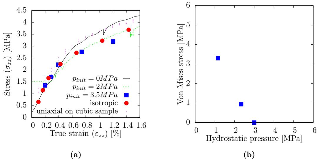
**Figure 3.26:** **a**-Stress-strain curve (parallel to master axis) for various initial pressure  $p_{init}$ . Responses are compared to an uniaxial test performed on a cubic sample. **b**-Yield stress versus the mean stress and the effective stress for various mean stresses.
