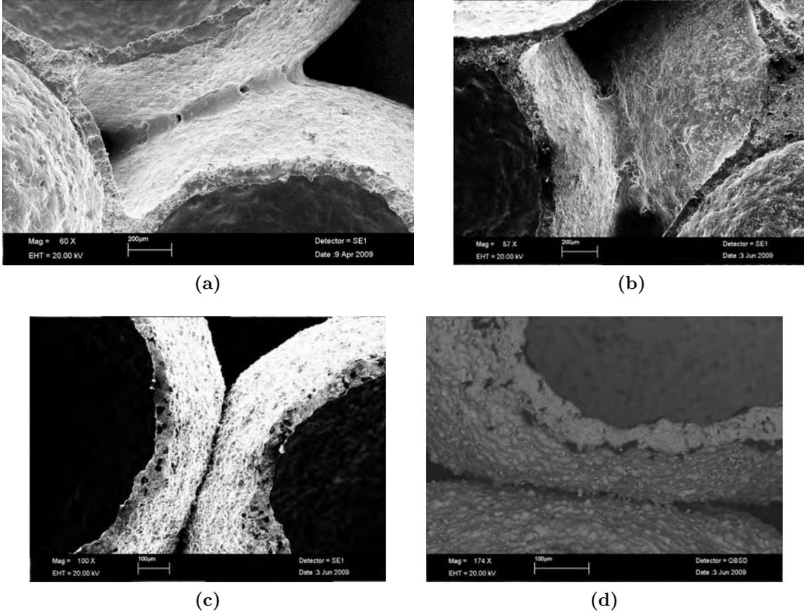
**Figure 1.3:** *S.E.M. images of the samples. Sandwich core material (a,b) can be compared to hollow spheres stackings that have not been integrated within a structure (c and d). Shapes of the necks are different.*
