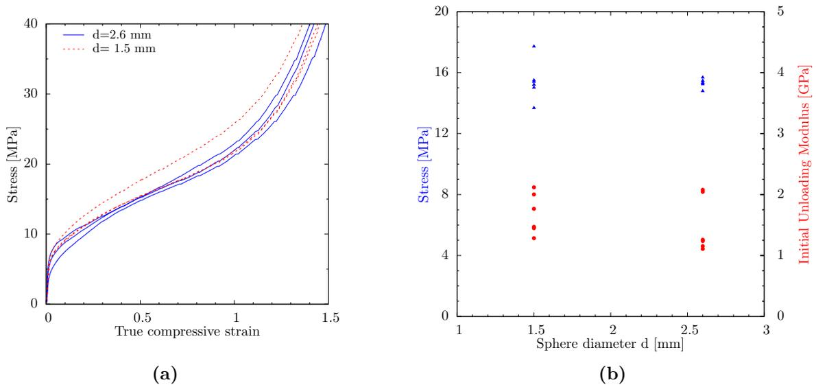
**Figure 3.5:** Influence of sphere size. **a**-Comparison of strain-stress curves. **b**-Comparison of extracted properties : stress at  $\epsilon = 50\%$  (upper points, blue triangles, with scale on the left hand side axis) and initial unloading modulus (lower points, red circles, with scale on the right hand side axis).
