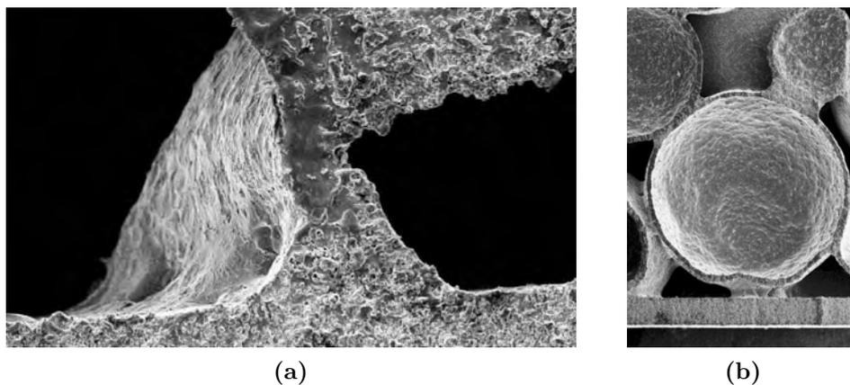
**Figure 4:** Overview of the brazing bonding with SEM. On the bottom of each picture can be seen a portion of a face of the sandwich structure. Scale have been varied, spheres have a radius size of 1.3 mm and shells a thickness of approximately 60  $\mu\text{m}$
