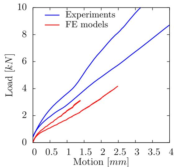
**Figure 3.13:** Comparison of the load-indentation curves for FE models and for experiments for two structures with faces of thickness 1 mm of core thickness of respectively 14 mm and 28 mm.
