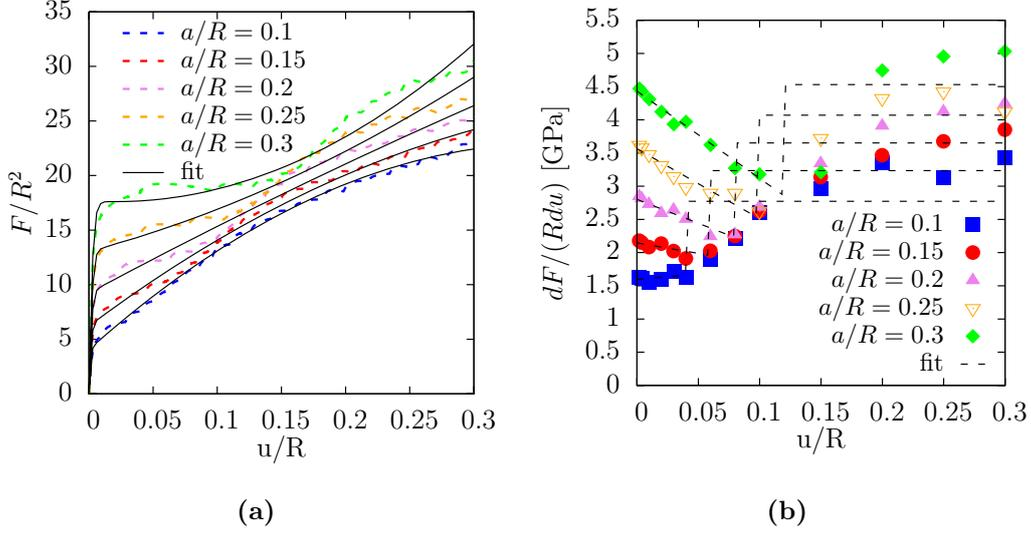
**Figure 2.3:** Simulations of 2 spheres of normalized shell thickness ( $t/R$ ) of 0.07 in compression. The size of the bonding ( $a/R$ ) has been varied. Simulations and corresponding model for the stress-strain curve (a) and for the unloading modulus evolution with strain (b).
