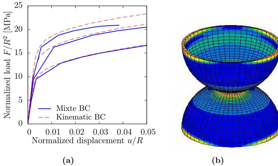
**Figure 2.7:** Comparison of the evolution of the normalized load  $F/R^2$  with the normalized displacement  $u/R$  for the shear loading of 3 necks (of normalized radius 0.1, 0.2 and 0.3) between two spheres of normalized shell thickness of 0.05 for respectively the full kinematic boundary condition and for a mixed kinematic-reaction boundary condition. The shape of the deformed mesh is presented for the model with kinematic-reaction boundary condition for a normalized neck size of 0.2.
