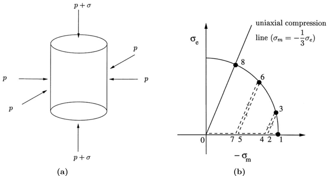
**Figure 3.4:** *Schematic of the loading state (a) and loading paths drawn on axes of effective stress versus mean stress (b) ( $\sigma_m = -(p + \frac{1}{3}\sigma$  and  $\sigma_e = -|\sigma|$ ) [Deshpande and Fleck, 2000].*
