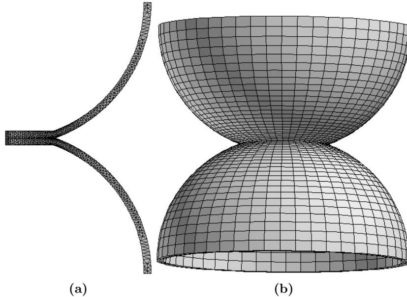
**Figure 3.9:** Meshes of the simulated bi-spheres. **a**-2D axi-symmetric mesh. **b**-3D mesh.
