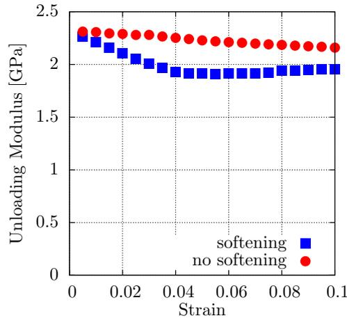
**Figure 2.11:** Evolution of the unloading modulus of a stacking with the strain. The sample contains 1000 particles and it is loaded in uniaxial compression with periodic boundaries conditions. The macroscopic behaviours with and without a local evolution of the contact stiffness are compared.
