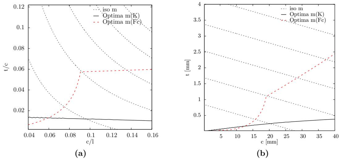
**Figure 1.10:** Location of sandwich structures with minimal weight for a constrain over the stiffness (solid black line) and for a constrain over the critical load (dashed red line). **a-** Axes are  $c/l$  and  $t/c$ . **b-** Axes are  $c$  and  $t$ .
