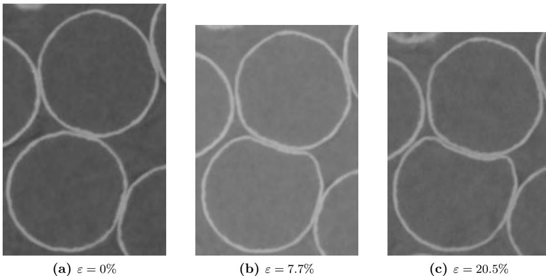
**Figure 4.1:** Indentation mechanism on hollow spheres observed thanks to X-ray tomography.
