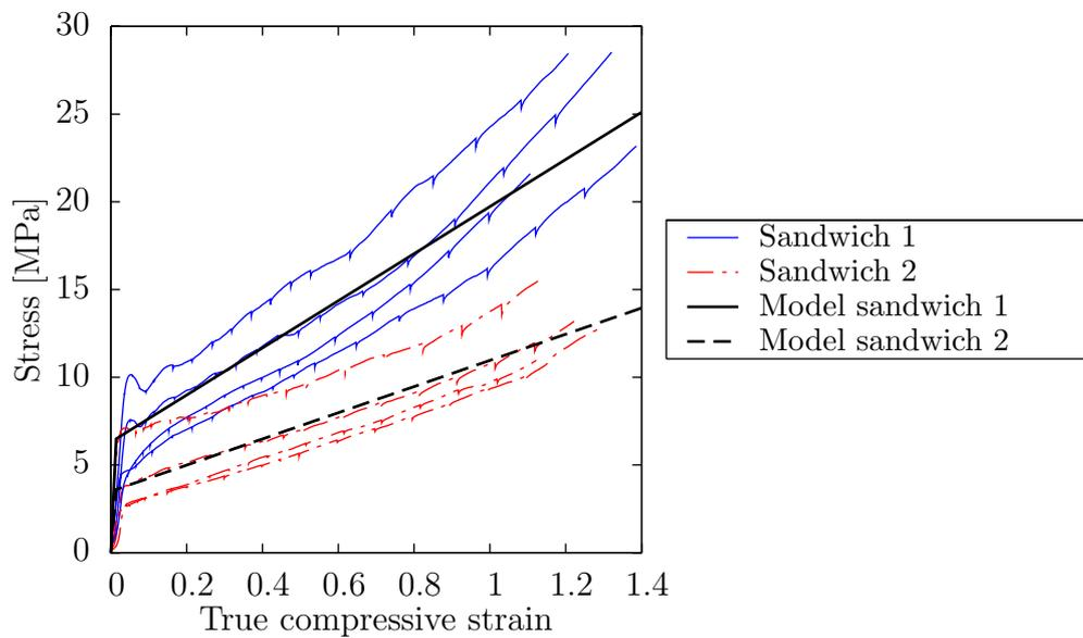
**Figure 1.10:** Compressive loading response and corresponding model. Depending on the core thickness  $c$  the model is varied.
