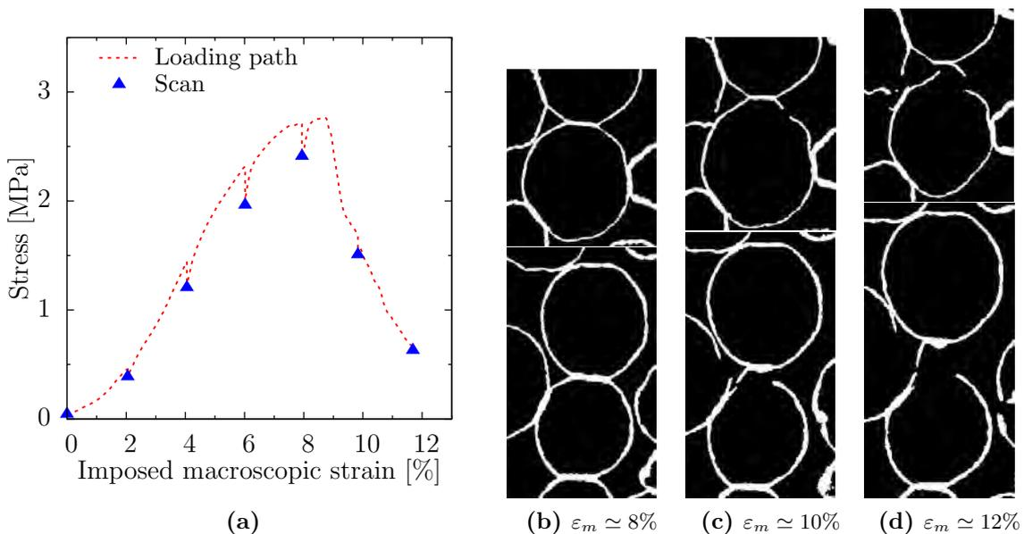
**Figure 3.20:** **a**-Position of the scans in a stress-strain map. **b,c,d**-With strain, damage increase by scratching of the shells. The strain  $\varepsilon_m$  presented is the macroscopic strain imposed by the machine, without any correction for the high compliance of the machine. The real average strain within the sample is almost 3 or 4 times smaller.
