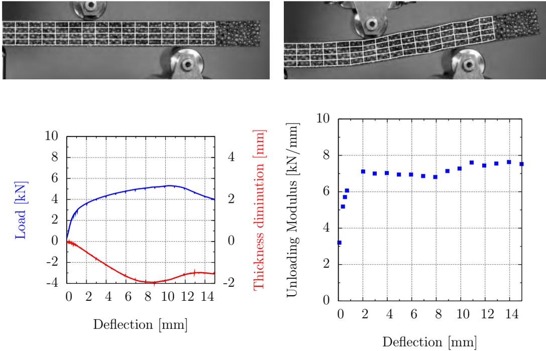
**Figure 2.9:** Digital image correlation of a part of a sandwich structures loaded in four points bending failing by face yield. Pictures were taken at deflection of 0mm, 2mm, 4mm, 8mm and 16mm. The grid points out the strain field within the core.
