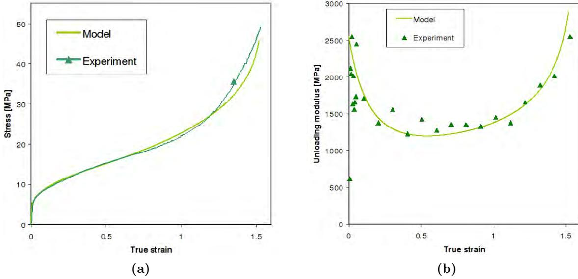
**Figure 4.11:** Model response for the stress-strain curve (a) and for the unloading modulus evolution with strain (b).
