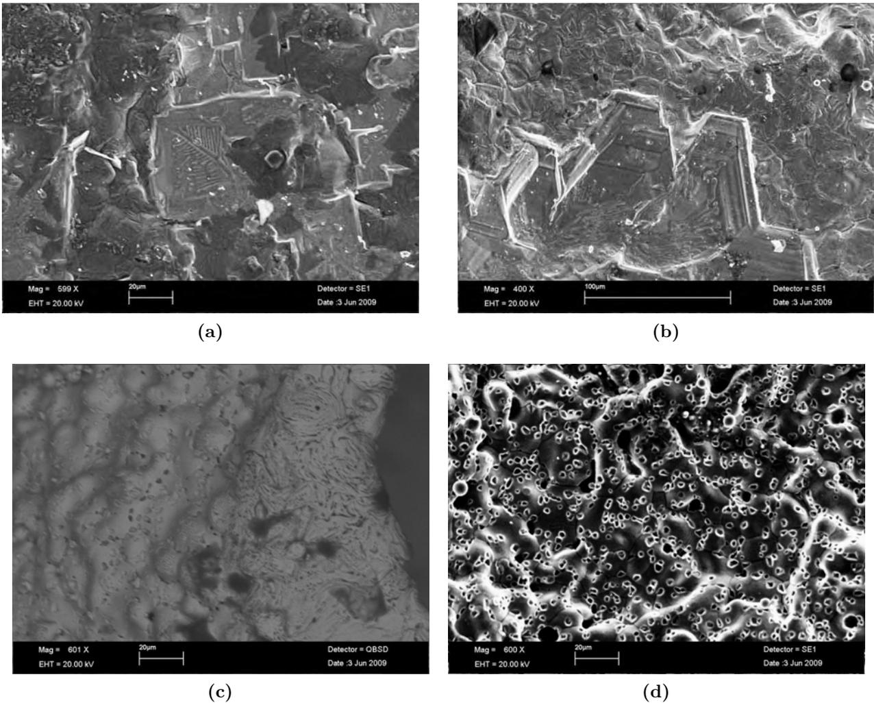
**Figure 1.2:** *S.E.M. images of the samples. Sandwich core material (a,b) can be compared to hollow spheres stackings that have not been integrated within a structure (c and d). Scatter of surfaces roughness is decreased but they are sharper. The microstructure of the constitutive material also seems to be changed.*
