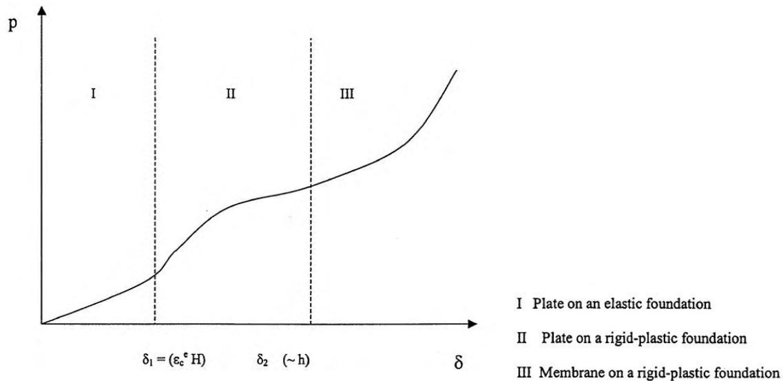
**Figure 1.11:** Depending on the depth of indentation three regimes can be identified for the upper face sheet [Fatt and Park, 2001].  $\epsilon_c^e$  is the core elastic limit,  $H$  is the core thickness and  $h$  is the face thickness.
