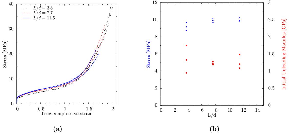
**Figure 3.3:** Influence of sample size. **a**-Comparison of strain-stress curves. **b**-Comparison of extracted properties : stress at  $\varepsilon = 50\%$  (upper points, blue triangles, with scale on the left hand side axis) and initial unloading modulus (lower points, red circles, with scale on the right hand side axis).
