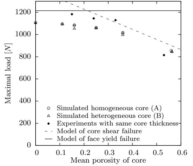
Fig. 6. Comparison of maximal loads.
