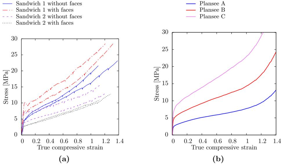
**Figure 1.8:** Compressive loading response. **a**-Stress-strain curves of the core material both with and without the sandwich structure faces. **b**-Stress-strain curves of the initial hollow spheres stackings of various densities.
