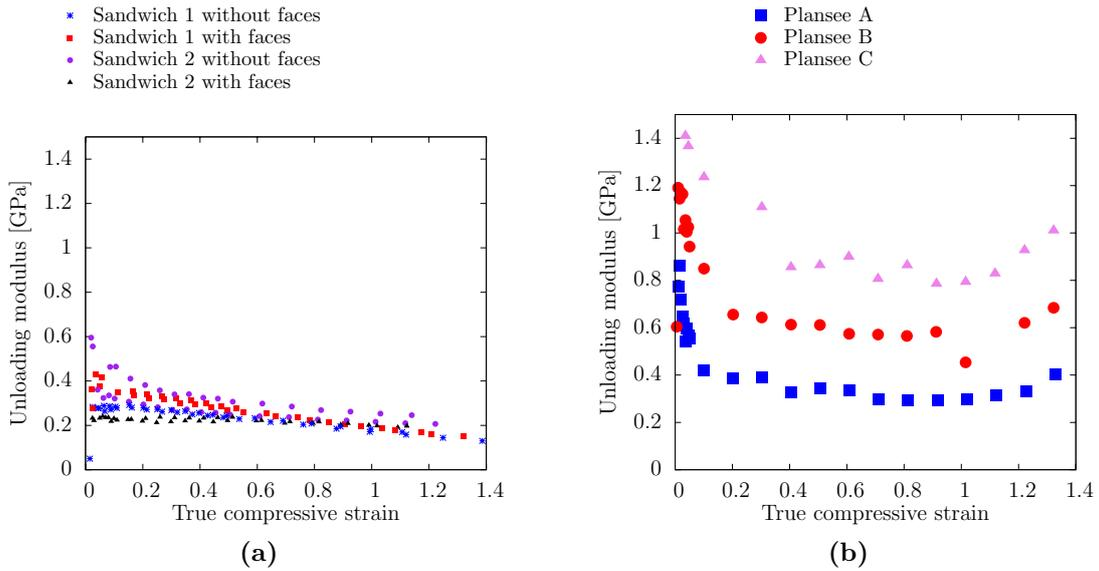
**Figure 1.9:** Compressive loading response. **a**-Unloading modulus evolution with strain for the core material both with and without the sandwich structure faces. **b**-Unloading modulus evolution with strain for the initial hollow spheres stackings of various densities.
