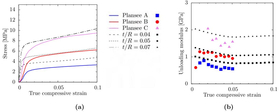
**Figure 3.12:** Confrontation of experiments and model for the stress-strain curves (a) and for the unloading modulus (b) under uniaxial compression with correction of both the shear contact law and the neck size.
