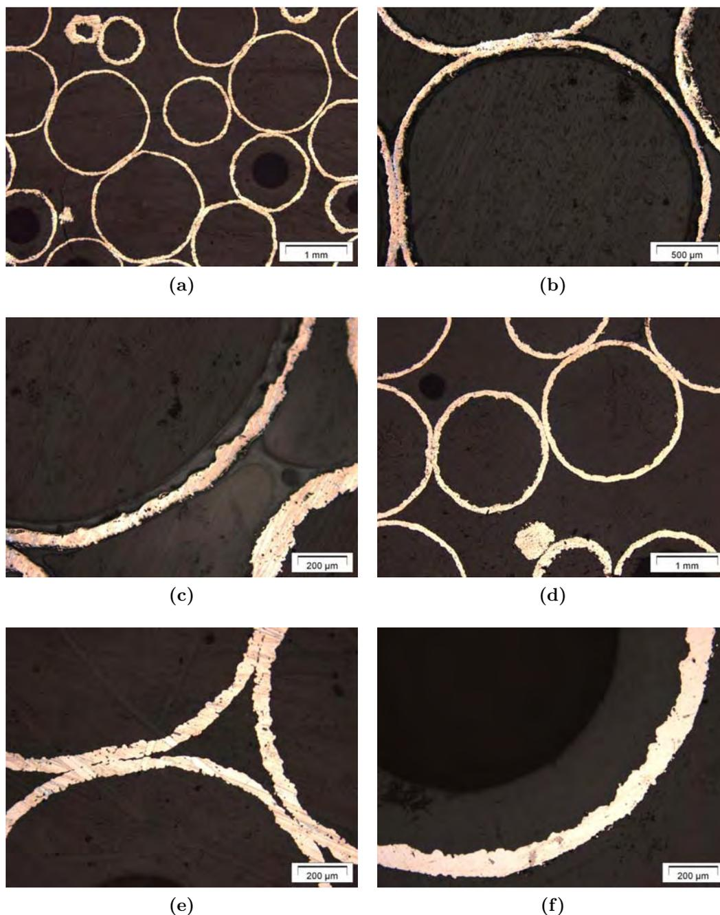
**Figure 1.2:** *Optical microscope observations of samples cold coated. One can see the variation of shell thickness within a single shell. Some severe defects can be observed (b). Mean shell thickness is different between top pictures (a,b,c) and bottom pictures (d, e,f). The roughness of interior surface and the rather smooth outer surface can be seen.*
