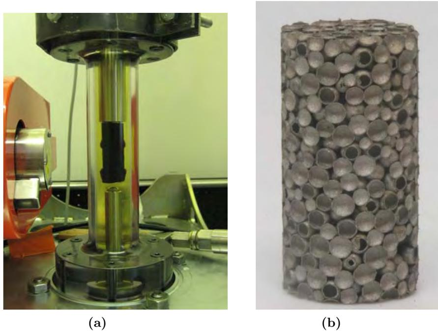
**Figure 3.5:** *a-Overview of the tri-axial pressure cell. b-Sample to be tested in the machine.*
