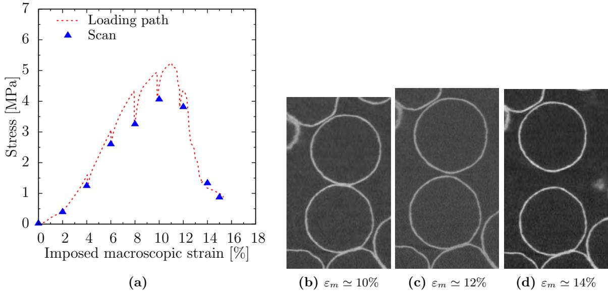
**Figure 3.21:** **a**-Position of the scans in a stress-strain map. **b,c,d**-With strain, the neck fails without damage for the shells. The strain  $\varepsilon_m$  presented is the macroscopic strain imposed by the machine, without any correction for the high compliance of the machine. The real average strain within the sample is almost 3 or 4 times smaller.
