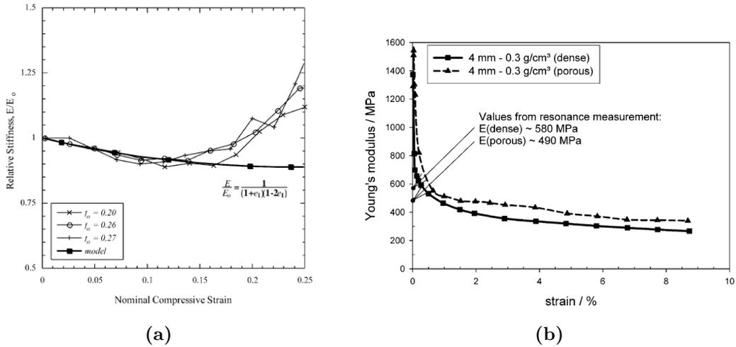
**Figure 2.11:** **a**-Unloading modulus evolution with strain of aluminum open cells foam under simple compressive loading [Marchi and Mortensen, 2001]. **b**-Same graph for hollow spheres stackings [Friedl et al., 2008].
