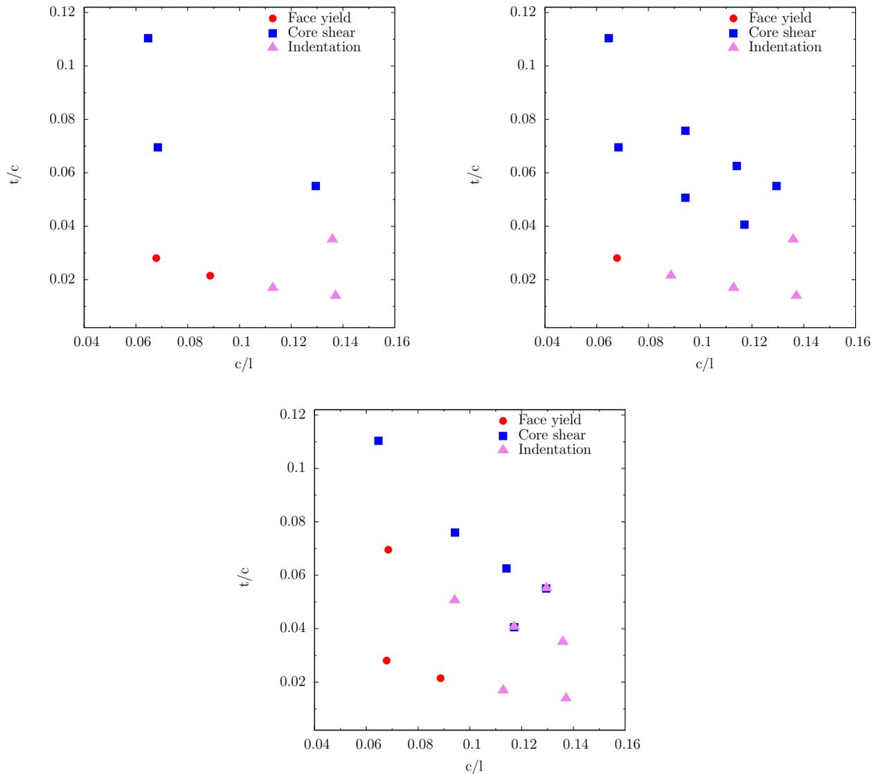
**Figure 2.16:** Failure maps of the normalized structure dimensions  $t/c$  and  $c/L$  for FE simulations (a), analytical models (b) and experiments (c).
