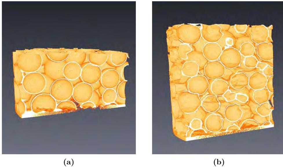
**Figure 1.6:** 3D visualisations of half sandwich structures with respectively thin core (a) and thick core (b). On the bottom, sandwich structure faces can be seen.
