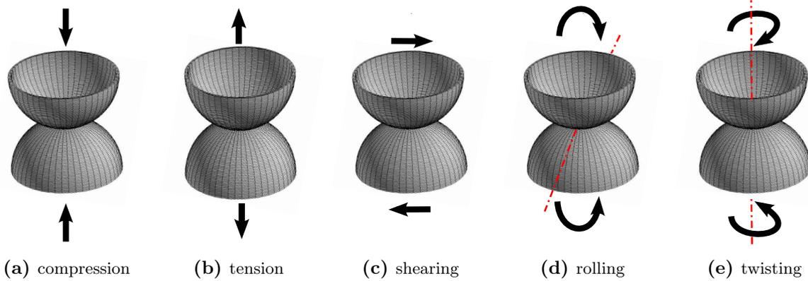
**Figure 2.1:** Loading conditions of the contact between 2 spheres.
