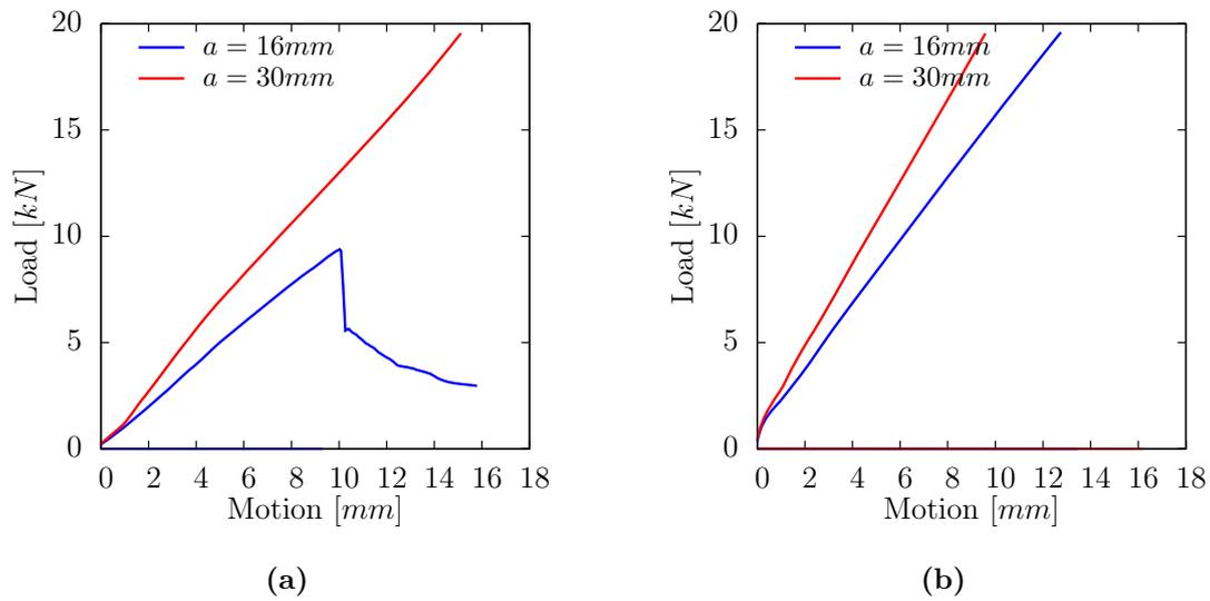
**Figure 3.9:** Load versus motion for two sandwich structures and for two indent sizes. **a-** Sandwich structure with face of 1 mm thickness. The indent prints are similar with both indent sizes. The larger the indent the smaller is the motion required to reach the maximal load. **b-** Sandwich structure with face thickness of 0.4 mm. With the small indent, the face fails by tearing, and thus the structure is perforated. The maximal load is never reached.
