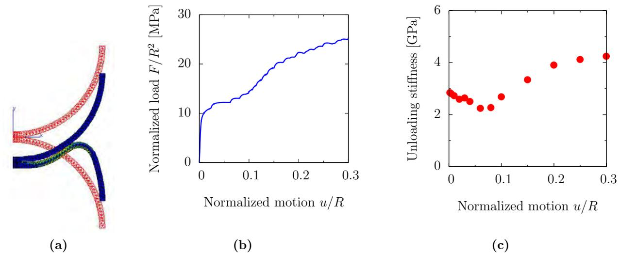
**Figure 2.2:** Simulations of 2 spheres of normalized shell thickness ( $t/R$ ) of 0.07 in compression. Axi-symmetric FEM has been used. **a**-Initial mesh (red) and deformed mesh (blue). **b**-Reaction on the upper face versus its motion. **c**-Evolution of the unloading stiffness with motion.
