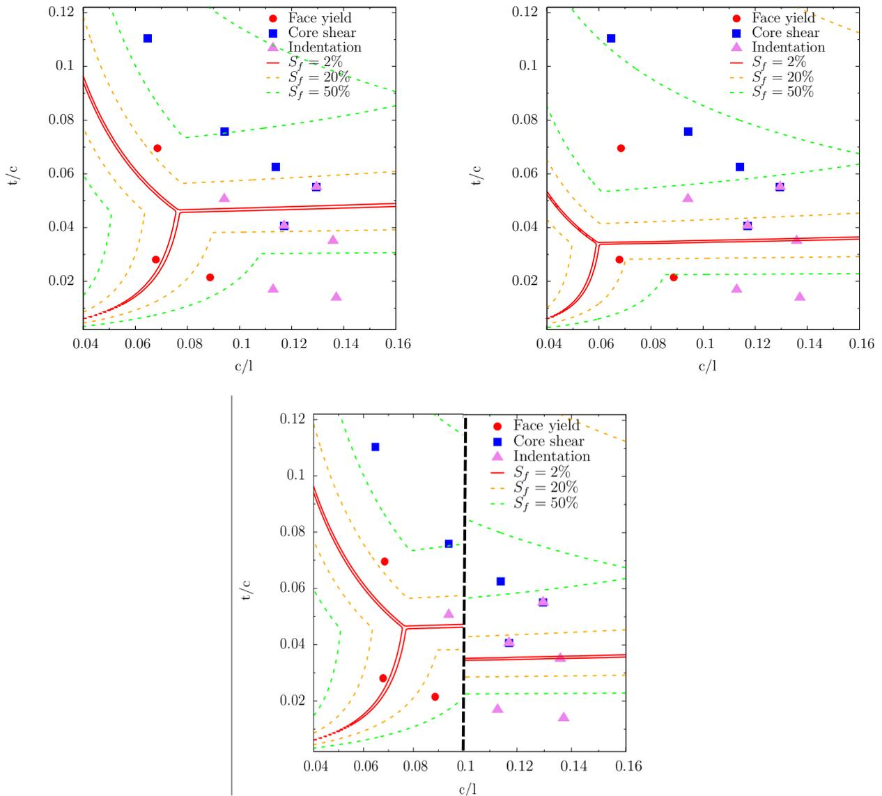
**Figure 2.17:** Failure maps of the normalized structure dimensions  $t/c$  and  $c/L$  for analytical models and experiments. **a**-The core is given an “high” yield stress (valid for thin cores). **b**-The core is given an “low” yield stress (valid for thick cores). **c**-Both previous map are combined in accordance to the relevant core thickness and core properties.
