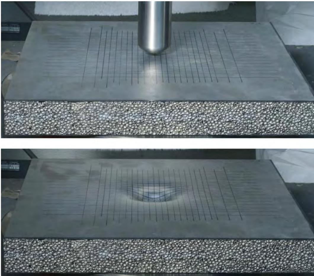
Figure 3.1: Sandwich plate just after an indent test. The indent has a diameter of 30mm.
