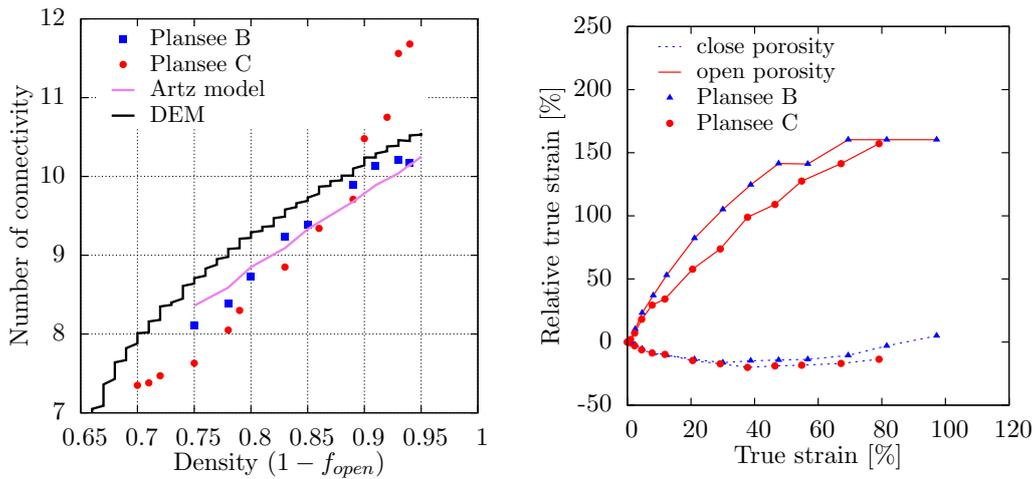
**Figure 4.8:** *a*-Evolution of the mean coordination number with the packing density. Artz model describes the re-organisation behaviour up to a mean coordination number of 10. *b*-Relative strain of open and closed porosity compared to the macroscopic strain. Most of the macroscopic strain is due to the open porosity.
