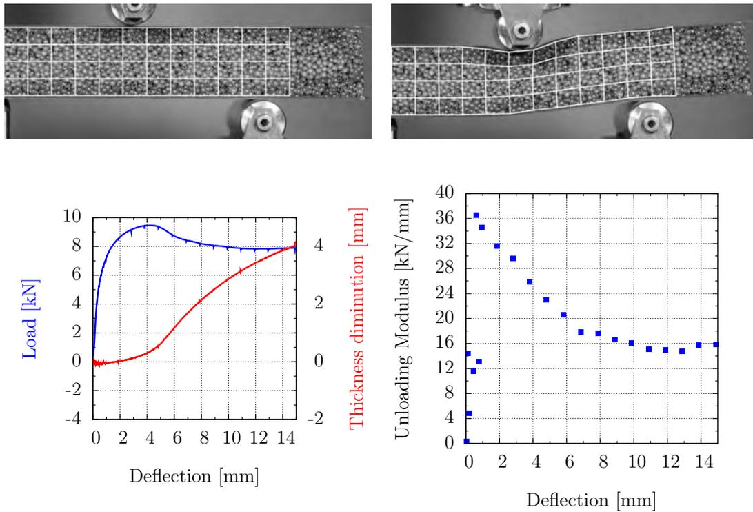
**Figure 2.10:** Digital image correlation of a part of a sandwich structures loaded in four points bending failing by indentation. Pictures were taken at deflection of 0mm, 2mm, 4mm, 8mm and 16mm. The grid points out the strain field within the core.
