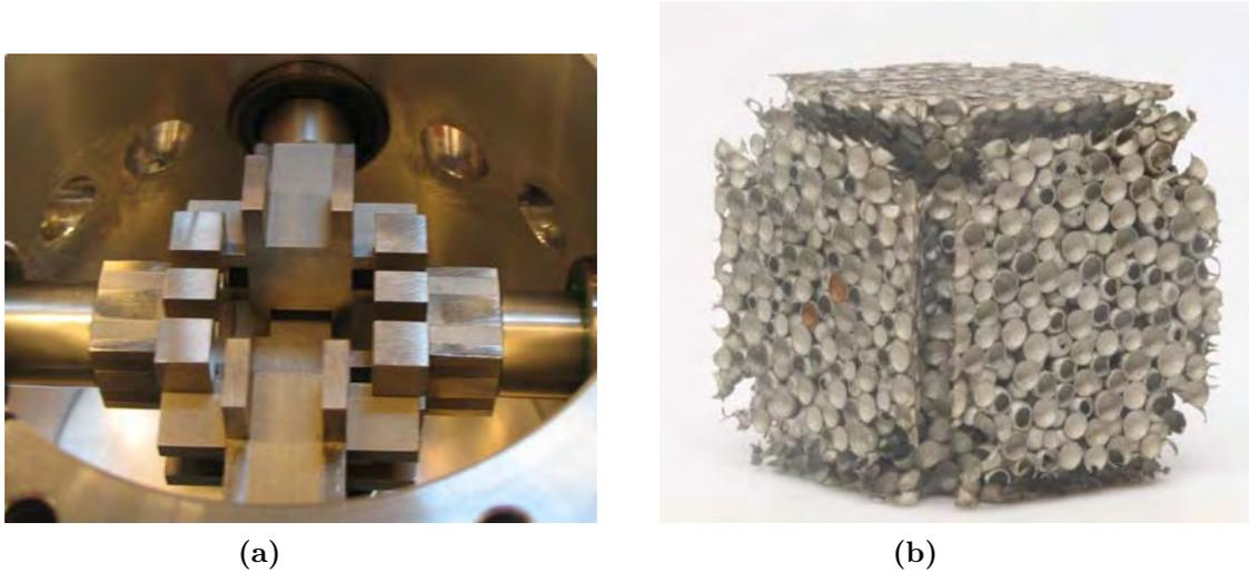
**Figure 3.3:** *a-Entangled plates of the multiaxial machine of EPFL. Upper plate has been removed for visibility. b-Sample to be tested in the machine.*
