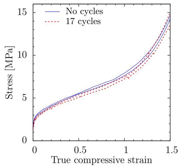
**Figure B.2:** *Stress-strain responses of samples enduring uniaxial compressive loading with or without loading-unloading sequences.*
