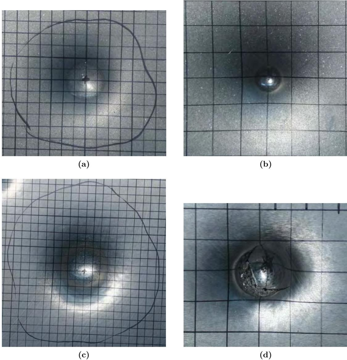
**Figure 3.8:** *Indent prints for two face thicknesses  $t$  and two indenter size (radius  $a$ ). **a**- $t = 1mm$ ,  $a = 15mm$ . **b**- $t = 1mm$ ,  $a = 8mm$ . **c**- $t = 0.4mm$ ,  $a = 15mm$ . **d**- $t = 0.4mm$ ,  $a = 8mm$ . The latter structure is perforated by the indenter. The face failed by excessive tensile strain. The grid is not consistent between the various plates.*
