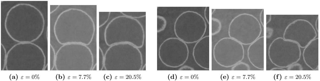
**Figure 2.7:** *a,b-Formation of a plastic ring in the upper shell under compressive loading. c-The plastic ring location changes and led to an indentation. d,e-Formation of a plastic ring in both shells under shear loading. f-The plastic ring locations do not change and thus symmetry is approximately kept.*
