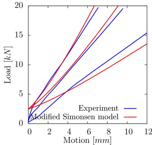
**Figure 3.7:** Comparison of the modeling of an perfectly-plastic membrane with modified yield stress clamped on a circle of 35mm of radius [Simonsen and Lauridsen, 2000] with contribution of the core and the experiments for a sandwich thickness of 28 mm and for varied face thickness.
