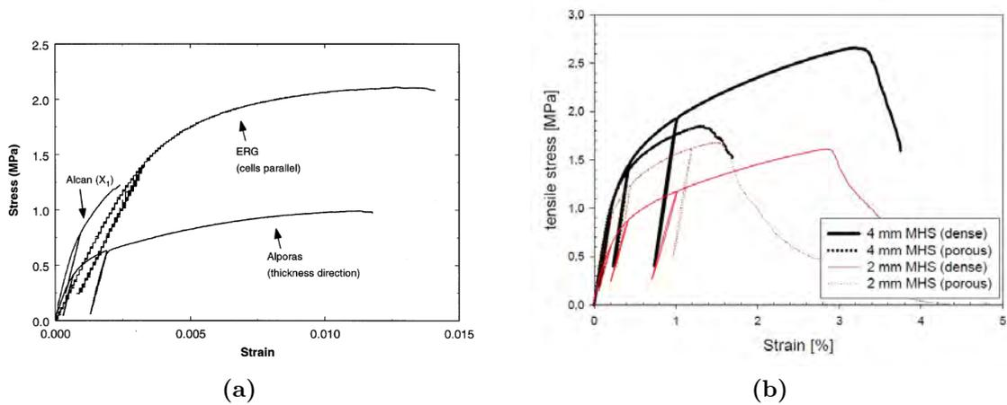
**Figure 2.12:** **a**-Tensile behavior of various aluminum foams [Andrews et al., 1999] **b**-Stress-strain curves of hollow spheres foams of a given density ( $\rho = 340\text{kg/m}^3$ ) with two spheres radius (2 and 4 mm) and two types of shells (dense or porous) under simple tensile loading [Motz et al., 2005]
