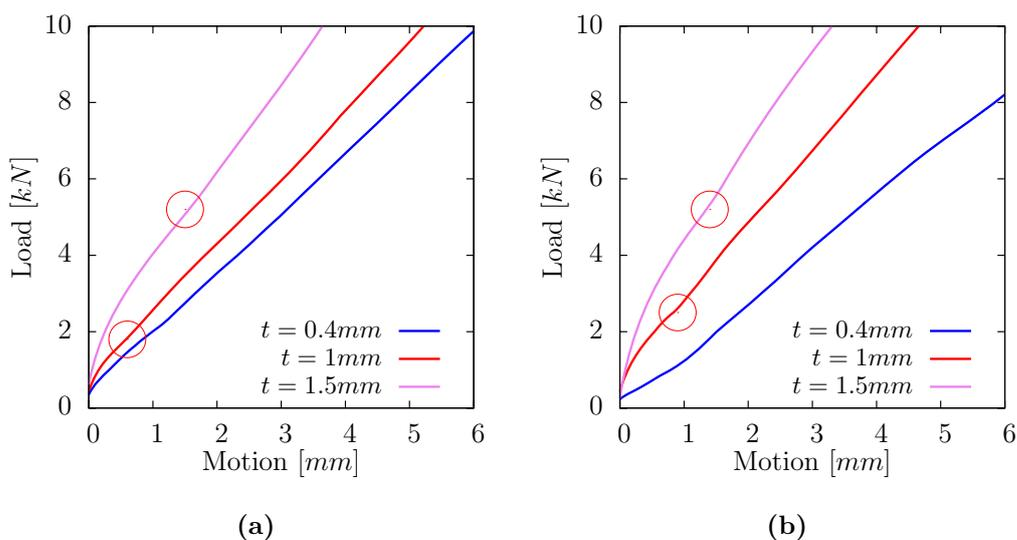
**Figure 3.3:** Transition between the plate and the membrane behaviour for sandwich thickness of respectively 24 mm (a) and 28 mm (b) for varied face thicknesses.
