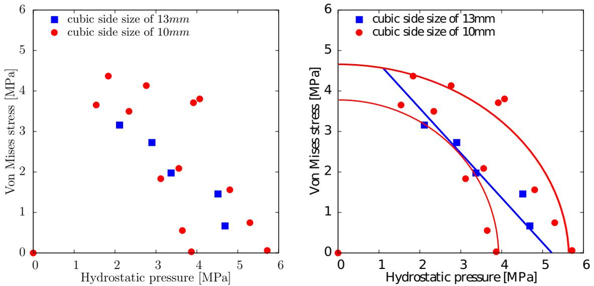
**Figure 3.23:** *Von Mises stress versus hydrostatic pressure elastic surface for samples with varied size. Models for the yield surface are proposed*
