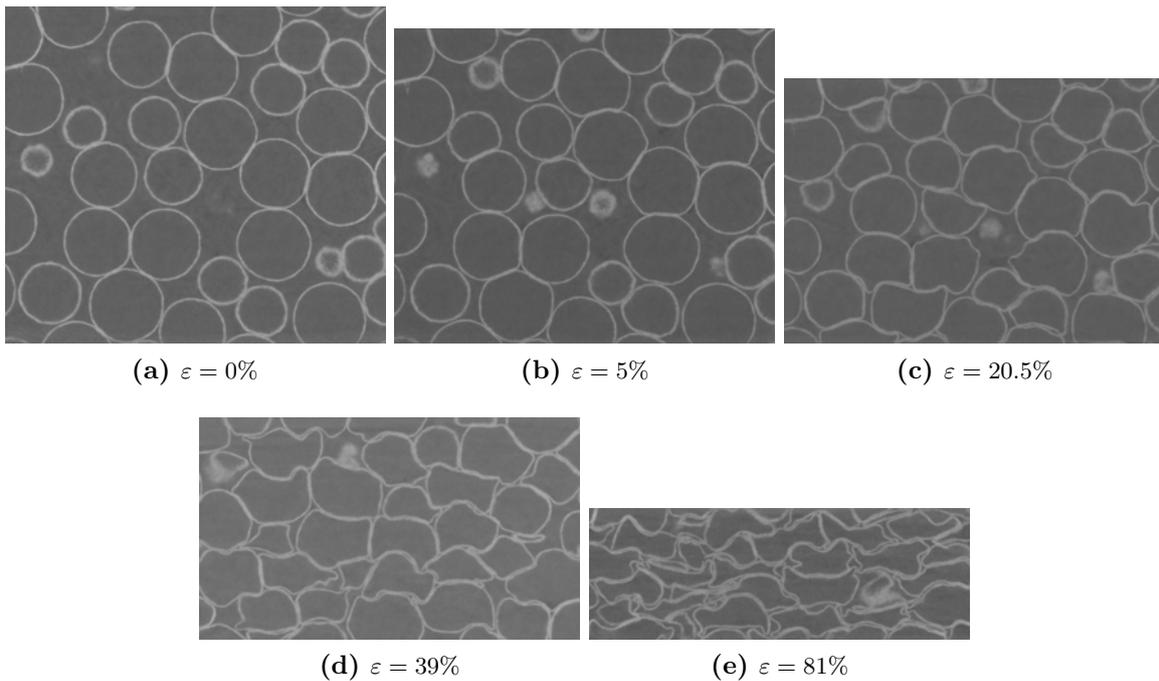
**Figure 4.9:** Tomography observation of a stacking during compression.
