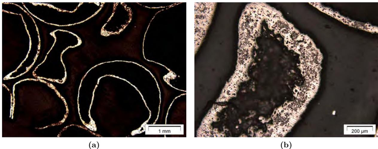
**Figure 1.1:** *Optical microscope observations of a sample hot coated. a-Pressure made cells to buckle. b-Porosity of the shell is important. The sharp inner surface can be guessed while one can see the rather smooth outer surface.*
