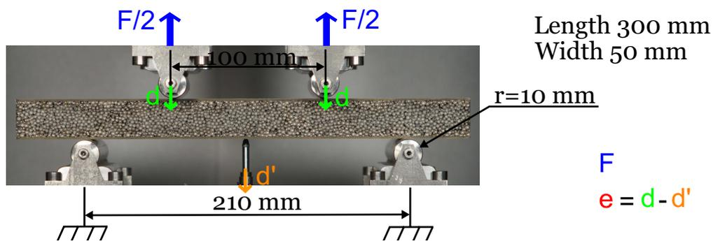
Figure 2.1: Dimensions and records of the four-points bending tests.
