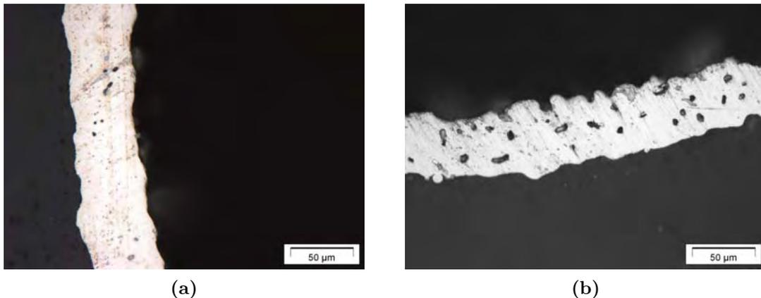
**Figure 1.1:** *Optical microscope observations of portions of shells. (a)-Shell of sandwich structure core material. The porosity is low and the characteristic length of surfaces roughness is large. (b)-Shell of a sphere that have not been integrated in a structure. Porosity is important and the surface is irregular.*
