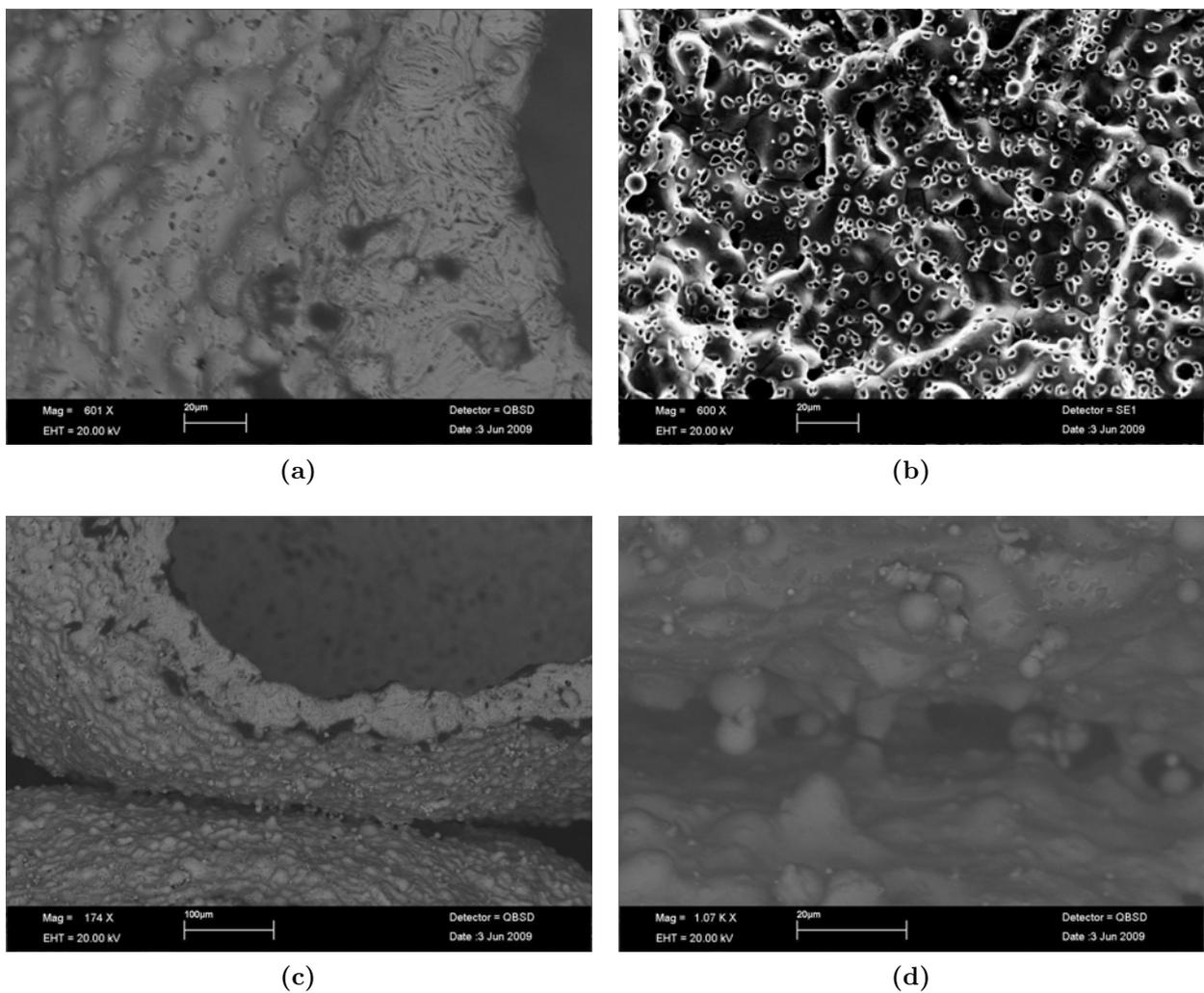
**Figure 1.3:** *S.E.M. images of the samples either with secondary electrons (b), either with back-scattered electrons (a,c,d). Cross section of the shell and roughness of outer surface can be observed (a). Shell microporosity is important (b). Sharp bonding between spheres is seen at various scales (c,d).*
