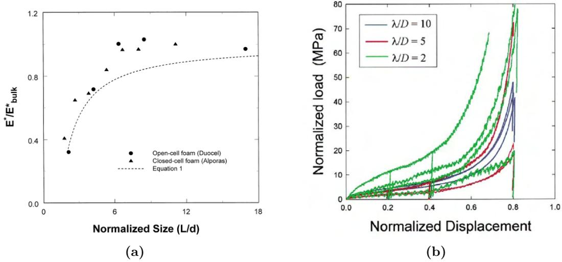
**Figure 2.14:** **a**-Evolution of the Young's modulus of open and closed foams with the sample size [Andrews et al., 2001]. **b**-Stress-strain curves of hollow spheres foams samples of various sizes under simple compressive loading ( $\lambda$  is the sample side size while  $D$  is the spheres diameter) [Lim et al., 2002]
