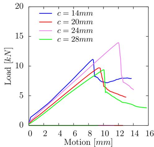
**Figure 3.10:** Load-indentation curves for sandwich structures with a face thickness of 0.4mm loaded with an indent of radius of 8mm. The fall down of the curves correspond to the perforation of the face.
