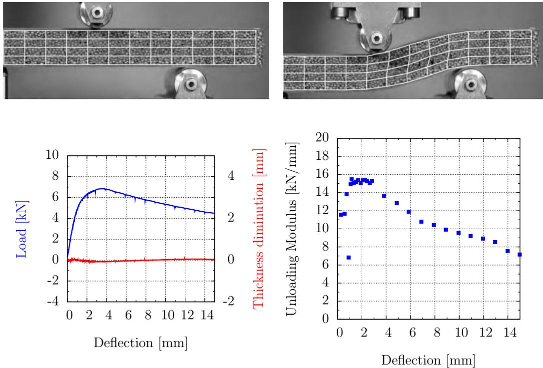
**Figure 2.8:** Digital image correlation of a part of a sandwich structures loaded in four points bending failing by core shear. Pictures were taken at deflection of 0mm, 2mm, 4mm, 8mm and 16mm. The grid points out the strain field within the core.
