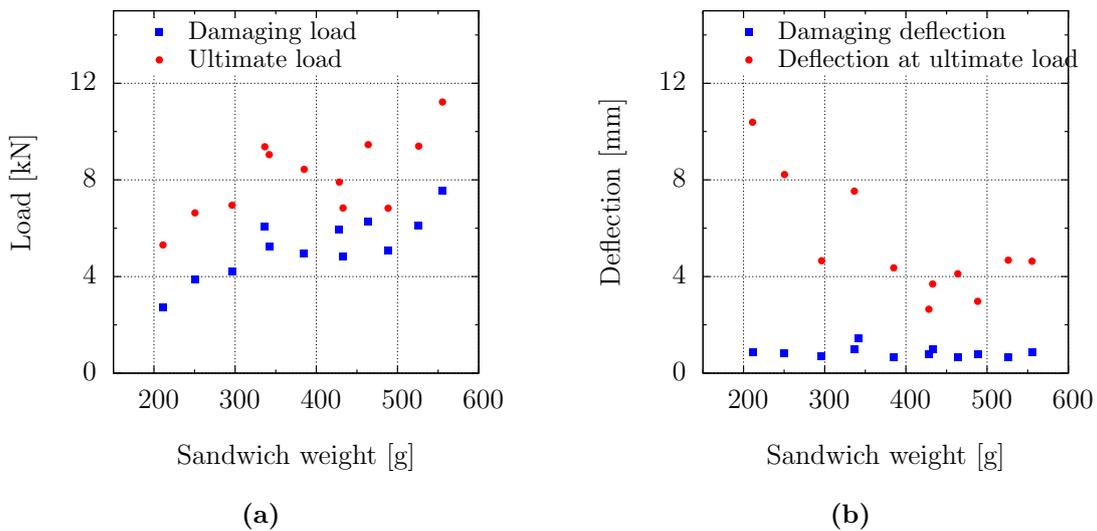
**Figure 2.3:** Characteristic loads (a) and associated deflections (b) plotted versus the weight of the sandwich structures.
