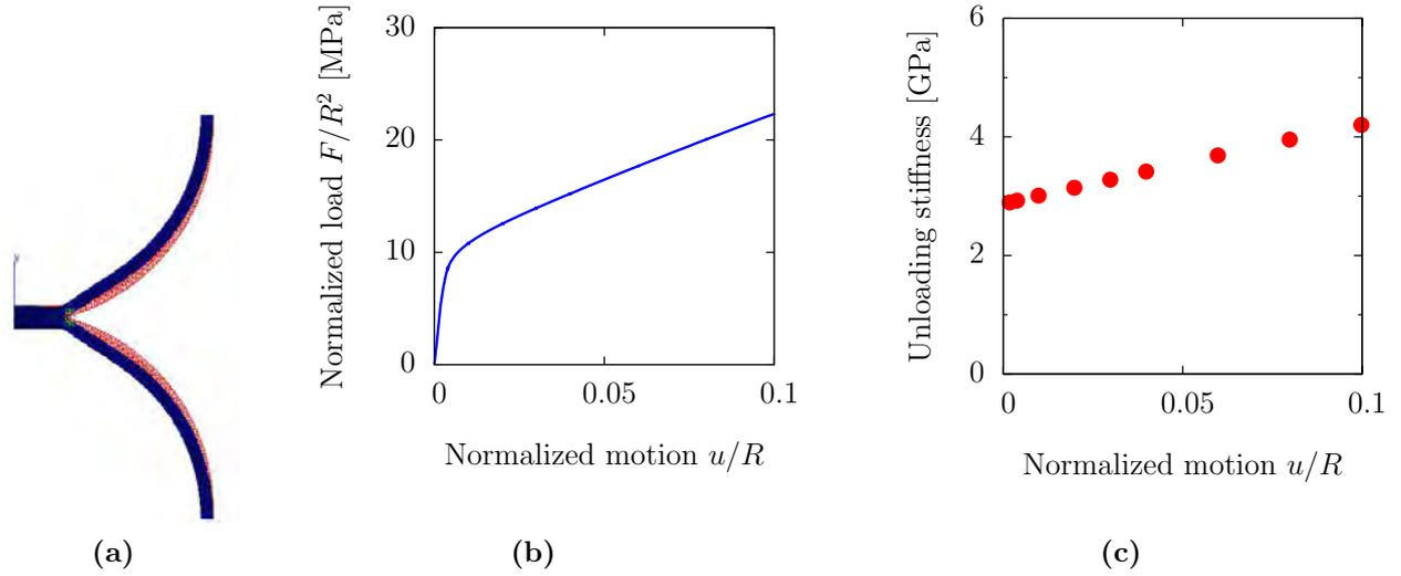
**Figure 2.4:** Simulations of 2 spheres of normalized shell thickness ( $t/R$ ) of 0.07 in tension. Axi-symmetric FEM has been used. **a**-Initial mesh (red) and deformed mesh (blue). **b**-Reaction on the upper face versus its motion. **c**-Evolution of the unloading stiffness with motions.
