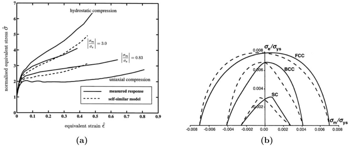
**Figure 2.13:** **a**-Influence of the loading path on aluminum foams behaviour [Deshpande and Fleck, 2000]. **b**-yield surface on axes of effective stress versus mean stress for various regular packings of hollow spheres [Sanders and Gibson, 2003a].
