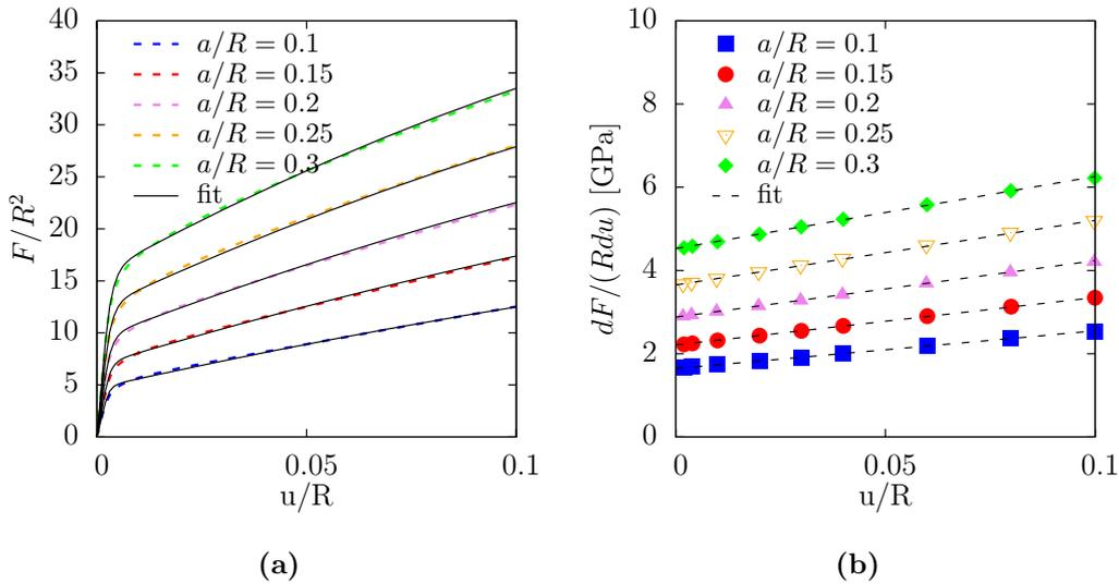
**Figure 2.5:** Simulations of 2 spheres of normalized shell thickness ( $t/R$ ) of 0.07 in tension. The size of the bonding ( $a/R$ ) has been varied. Simulations and corresponding model for the stress-strain curve (**a**) and for the unloading modulus evolution with strain (**b**).
