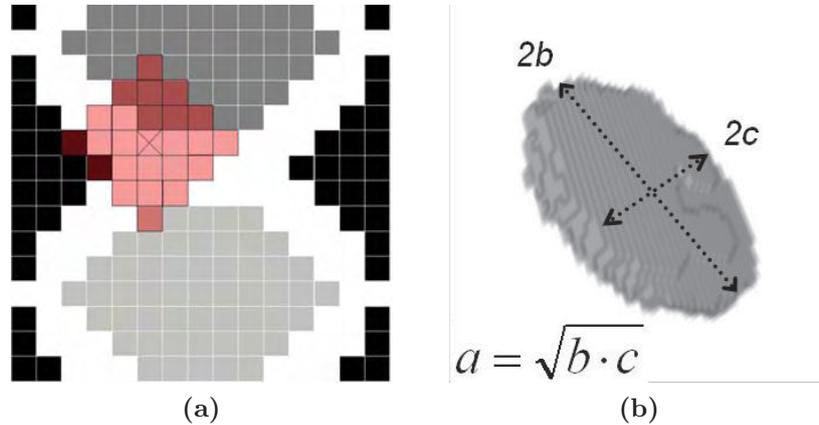
**Figure 1.8:** Neck detection and measure. **a**-A pattern is moving on the shell. When it intercepts two spheres interior its center is within a neck. **b**-Estimation of the neck diameter based on the two larger axes of an ellipsoid.
