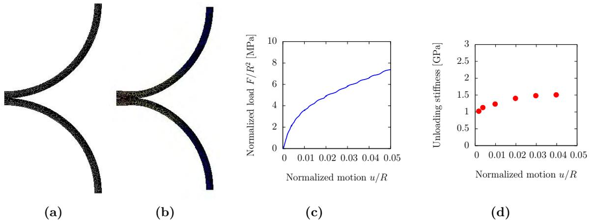
**Figure 2.9:** Simulations of 2 non connected spheres of normalized shell thickness ( $t/R$ ) of 0.07 in compression. Axi-symmetric FEM has been used. **a**-Initial mesh. **b**-Deformed mesh. **c**-Reaction on the upper face versus its motion. **d**-Evolution of the unloading stiffness with motions.
