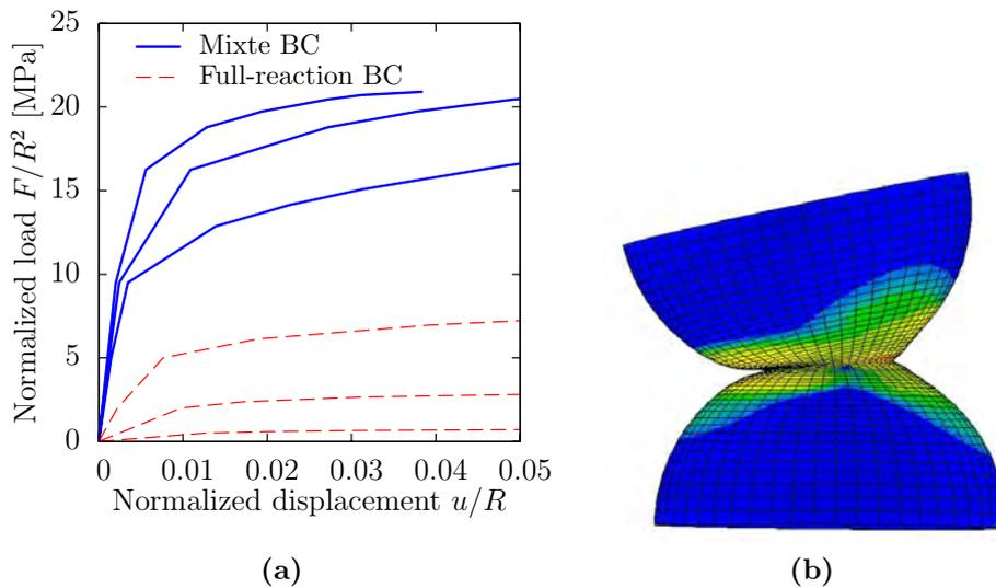
**Figure 2.8:** Comparison of the evolution of the normalized load  $F/R^2$  with the normalized displacement  $u/R$  for the shear loading of 3 necks (of normalized radius 0.1, 0.2 and 0.3) between two spheres of normalized shell thickness of 0.05 for respectively the mixed kinematic-reaction boundary condition and for a full reaction boundary condition. The shape of the deformed mesh for the full-reaction boundary conditions is presented for a normalized neck size of 0.2.
