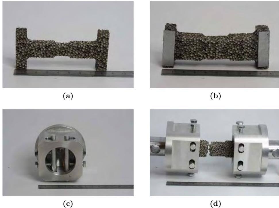
**Figure 3.2:** *a-Tensile specimen of cubic working volume of 10 mm side size before reinforcement of the heads. b-Tensile specimen of cubic working volume of 20 mm side size after test. c-Top view of one part of the tensile system (Screws are used to fix the rollers span). d-Front view of the tensile system with a specimen after failure.*
