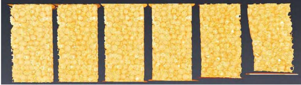
**Figure 3.25:** Sample loaded in compression parallel the cylinder axis with a confinement pressure of 1MPa. The section shows how buckling is initiated by strain localization (on the left side, a third of the height approximately).
