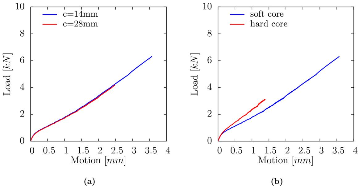
**Figure 3.12:** a-Load-indentation curves of FE models for two identical structures if not for the core thickness that is respectively of 14 mm and 28 mm. b-Load-indentation curves of FE models for two identical structures if not for the core material that is either hard or soft.
