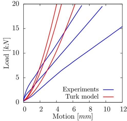
**Figure 3.4:** Comparison of the modeling of an elastic membrane resting on a rigid-plastic foundation [Türk and Fatt, 1999] and the experiments for a sandwich thickness of 28 mm and for varied face thickness.
