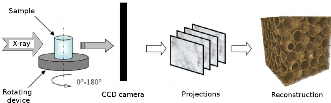
**Figure 3.6:** *Overview of the principle of X-ray tomography.*
