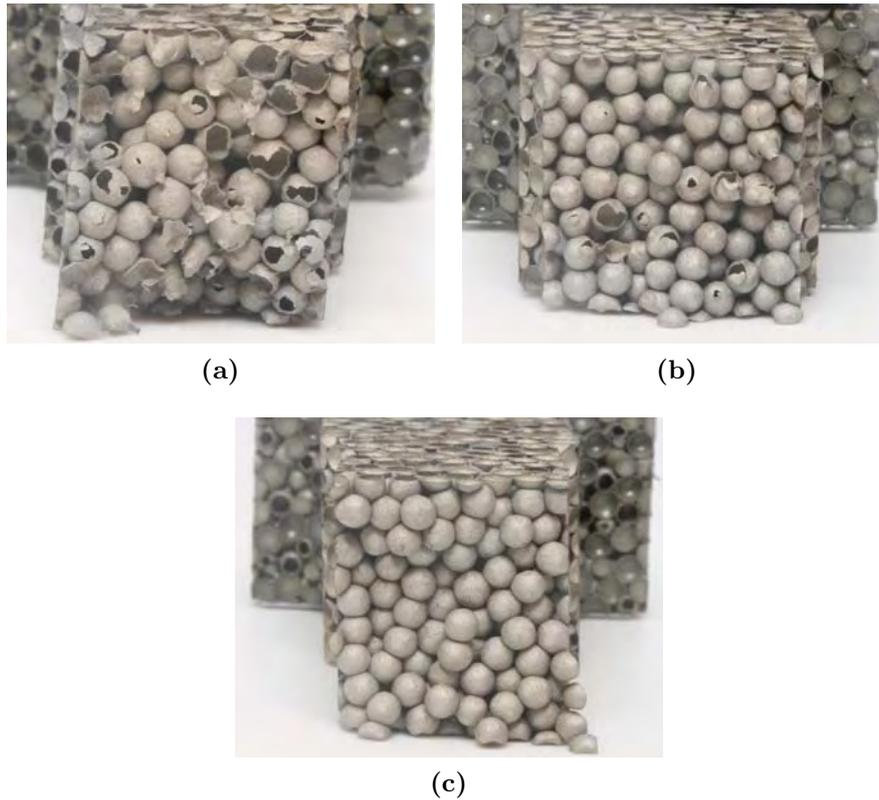
**Figure 3.18:** *Influence of foam density. a-For thin shells, failure occurs in the shell. b-For medium shell thickness, there is a partition between the failure in the neck and in the shells. c-For thick shells, failure occurs in the neck without any damage for the shells.*
