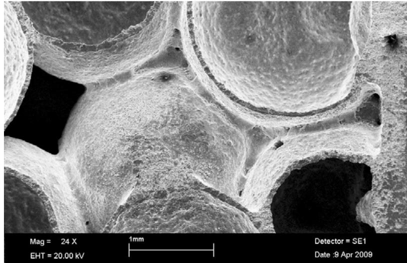
**Figure 1.4:** SEM observation of the core material at the vicinity of the sandwich structure face. On the right hand side, the face of the sandwich structure is visible. The brazing element spreads within the core over a length of several spheres diameters.
