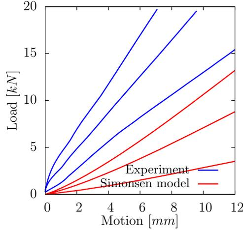
**Figure 3.6:** Comparison of the modeling of an perfectly-plastic membrane clamped on a circle of 35mm of radius [Simonsen and Lauridsen, 2000] and the experiments for a sandwich thickness of 28 mm and for varied face thickness.
