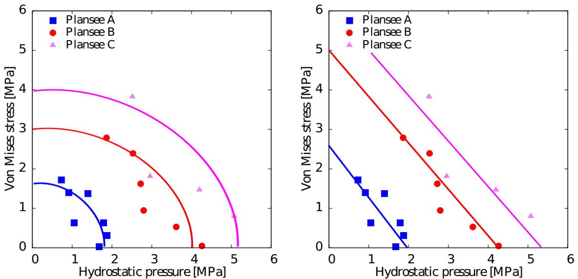
**Figure 3.24:** *Von Mises stress versus hydrostatic pressure elastic surface for samples with varied density. The shape of the yield surface is proposed.*
