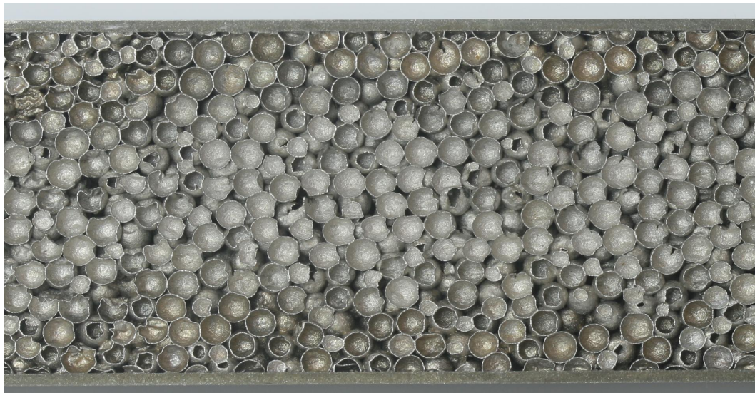
Figure 1.7: Cross section of a sandwich structure. The core varies depending on its distance to the faces
