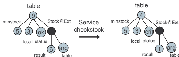
Figure 2: Our sample document after the materialization of the call to Checkstock . The initial result of Stock@Ext is 6, which means that there are more than 5 tables (6 in factory+3 local) hence the status is ok. The next check reports that the number of tables in the factory is 1, hence there are less than 5 tables and the critical status is triggered. Next, an order for table will be sent to the factory.
