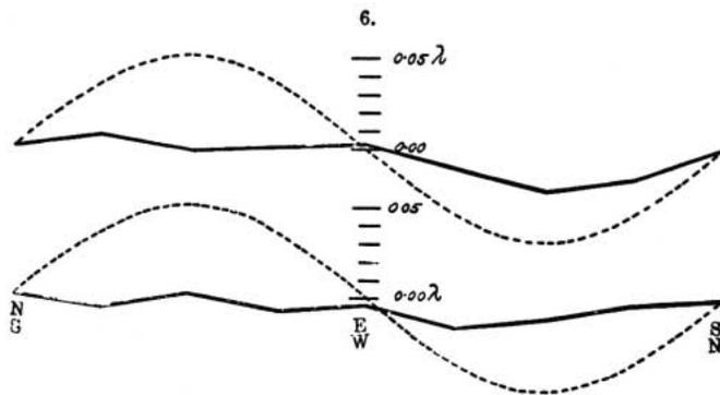
placement due to the relative motion of the earth and the luminiferous ether, this cannot be much greater than 0.01 of the distance between the fringes. Considering the motion of the earth in its orbit only, this
