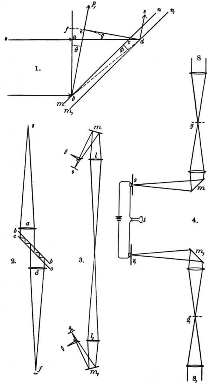
would be about one-millionth of the original intensity, so that if sunlight or the electric arc were used it could still be readily seen. The mirrors *bb*, and *cc*, would differ from parallelism sufficiently to separate the successive images. Finally, the apparatus need not be mounted so as to revolve, as the earth's rotation would be sufficient.
