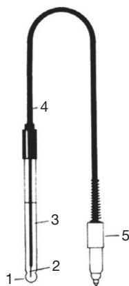
Figure 1 Typical commercial glass membrane electrode. (1) sensitive glass membrane; (2) Ag/AgCl internal reference electrode; (3) internal solution with constant pH; (4) cable; (5) plug.
