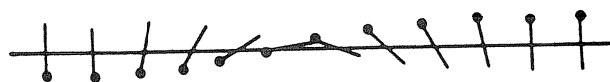
Fig. 10.3. Pegs on a line representing the kink (soliton) solution to the sine-Gordon equation.
