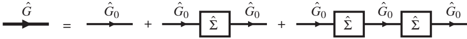
Fig. 5.4 Diagrammatic series for the dressed Green function \hat{G} , rearranged into the Dyson series. The self-energy blocks contain the sum of all irreducible diagrams.
