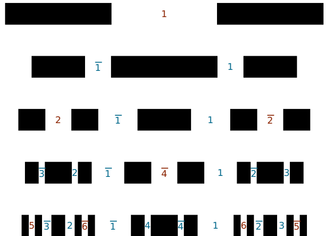
Figure 9: The gap labels, q , of the first few approximants. Blue: stable gaps, red: transient gaps. All the stable gaps are iterates of the 2 main gaps, while all the transient gaps are the iterates of the E = 0 gap.
