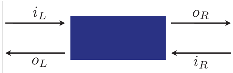
Figure 1.1. Schematic description of the scattering matrix setup, showing the incoming ( i_R, i_L ) and outgoing ( o_R, o_L ) amplitudes on the left and right of the scattering region.
