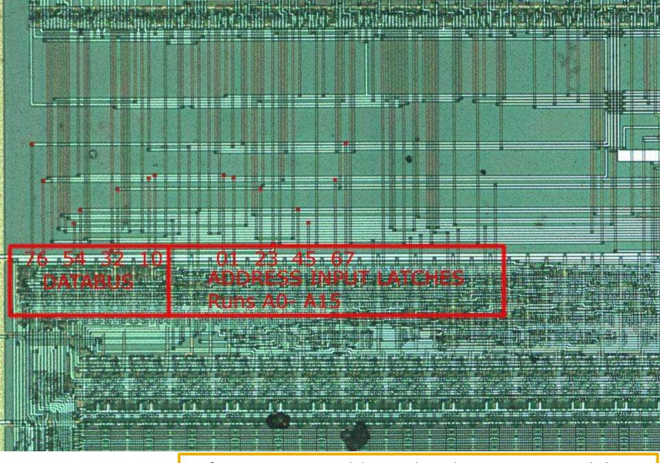
Infineon SLE66 address/data bus, courtesy Flylogic
