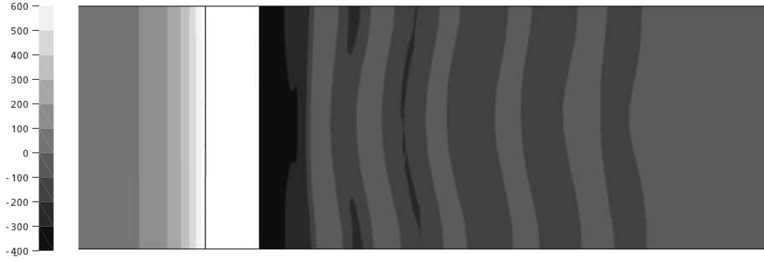
Figure 12: Pressure field on the vertical plane through the cylinder axis parallel with the inlet flow direction at t = 7.9 s.
