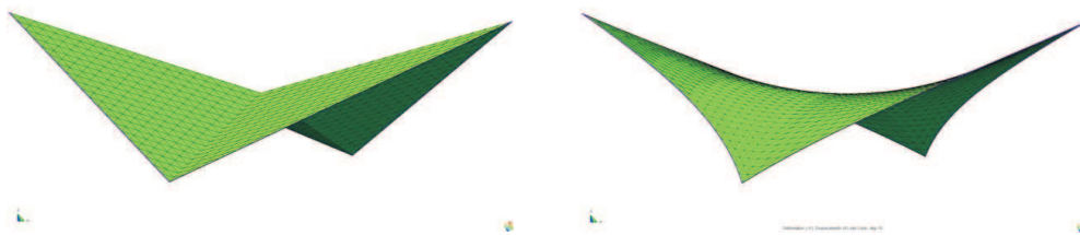
Figure 12: Initial and converged configuration of form finding of four point tent
