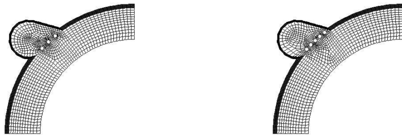
Figure 5: Deformed mesh for steady configuration with stents: 3 stents (left) and 5 stents (right).
