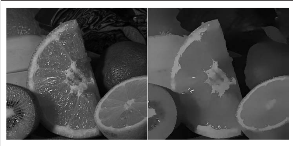
Figure 9-11. Mean-shift segmentation over scale using cvPyrMeanShiftFiltering() with parameters max_level=2 , spatialRadius=20 , and colorRadius=40 ; similar areas now have similar values and so can be treated as super pixels, which can speed up subsequent processing significantly
