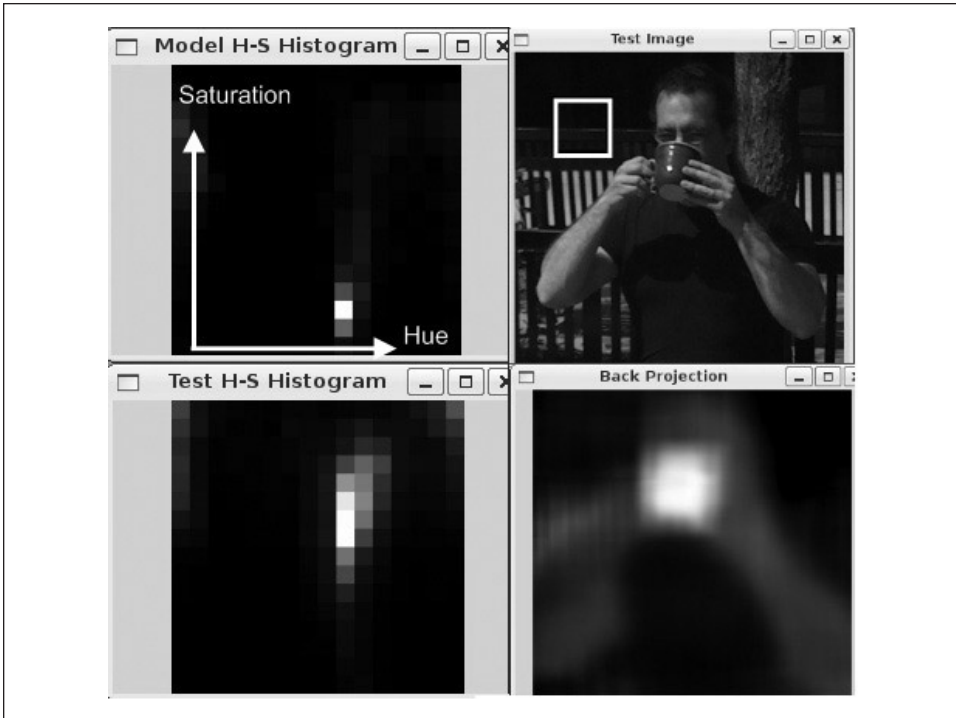
Figure 7-9. Using cvCalcBackProjectPatch() to locate an object (here, a coffee cup) whose size approximately matches the patch size (white box in upper right panel): the sought object is modeled by a hue-saturation histogram (upper left), which can be compared with an HS histogram for the image as a whole (lower left); the result of cvCalcBackProjectPatch() (lower right) is that the object is easily picked out from the scene by virtue of its color
