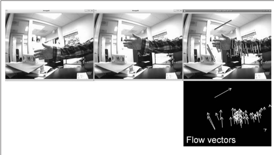
Figure 10-10. Sparse optical flow from pyramid Lucas-Kanade: the center image is one video frame after the left image; the right image illustrates the computed motion of the “good features to track” (lower right shows flow vectors against a dark background for increased visibility)
