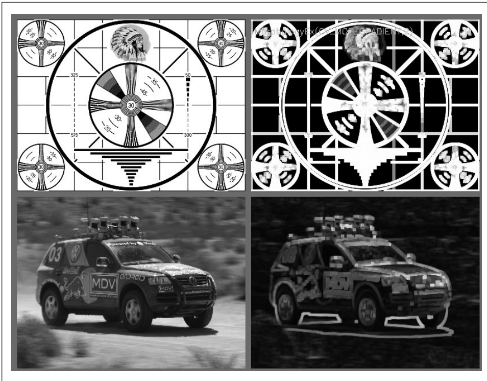
Figure 5-15. Results of the morphological gradient operator: bright perimeter edges are identified
