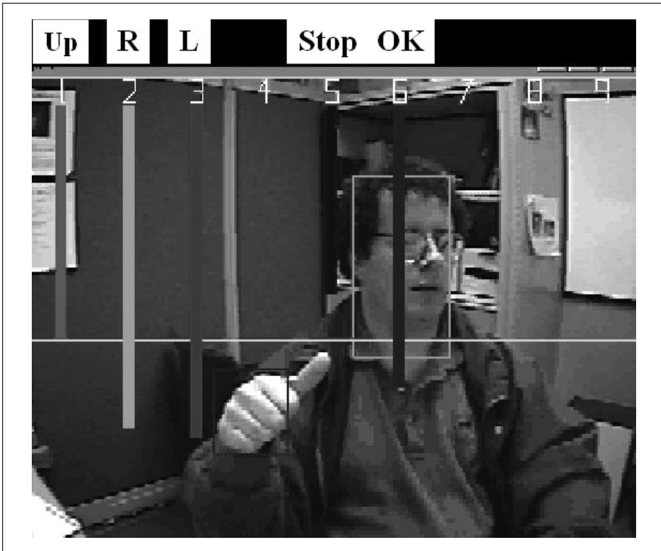
Figure 7-1. Local histograms of gradient orientations are used to find the hand and its gesture; here the “winning” gesture (longest vertical bar) is a correct recognition of “L” (move left)
