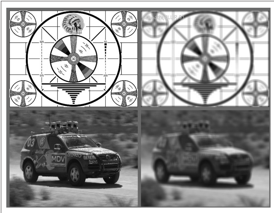
Figure 5-1. Image smoothing by block averaging: on the left are the input images; on the right, the output images
