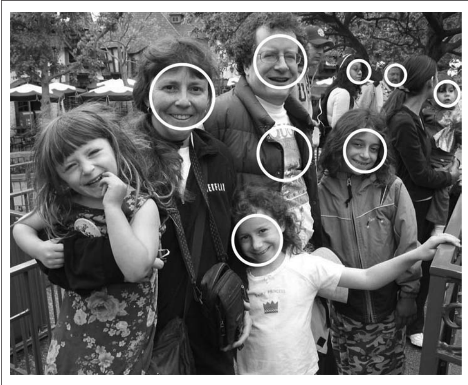
Figure 13-16. Face detection on a park scene: some tilted faces are not detected, and there is also a false positive (shirt near the center); for the 1054-by-851 image shown, more than a million sites and scales were searched to achieve this result in about 1.5 seconds on a 2 GHz machine
