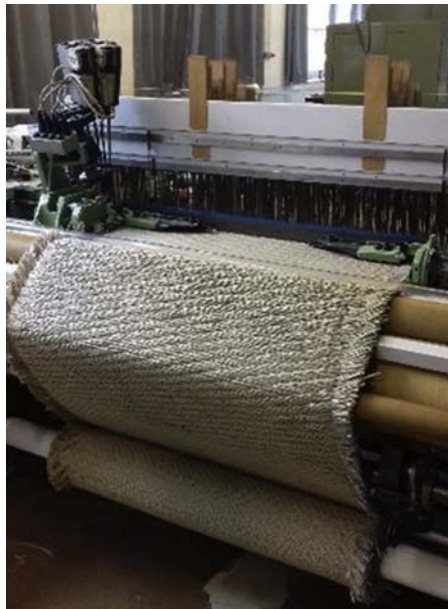
Figure 5.12 Manufacture of 3D-warp interlock from flax rovings at Gemtex-Lab.
