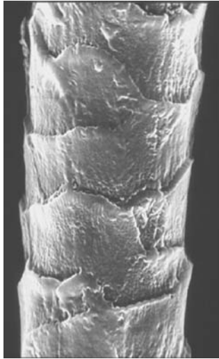
Figure 8.10 Scanning electron micrograph of wool fibre treated with chlorine/Hercosett.
