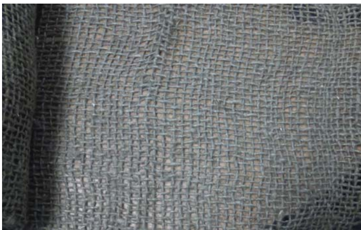
Figure 5.14 Textile tow woven geotextile.
