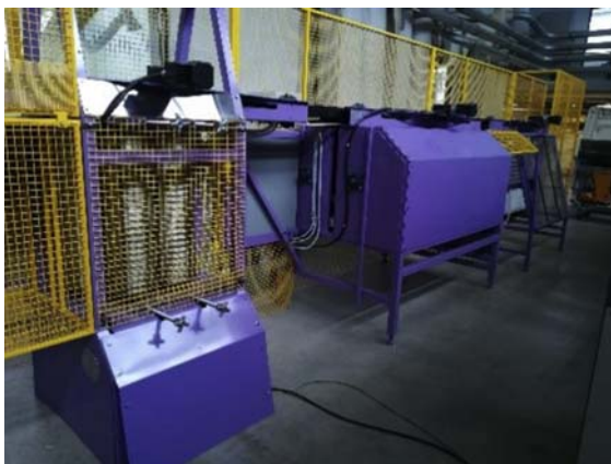
Figure 5.3 Laboratory scutching and hackling device from TAP-ROOT FIBRE LAB (ENI of Tarbes-France).
