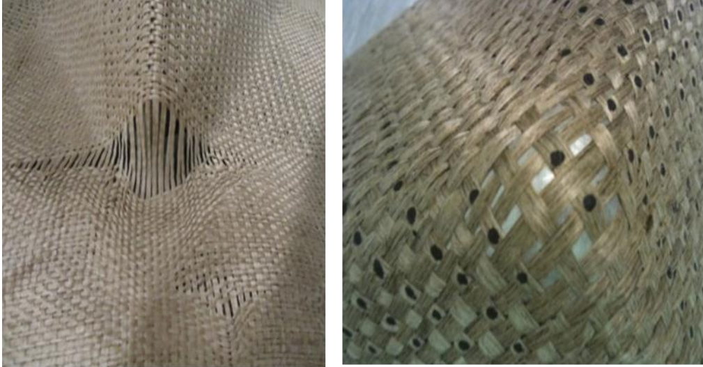
FIGURE 1. Tow sliding defect during complex shape forming of flax plain weave fabric
