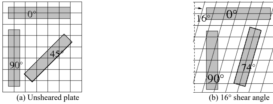
FIGURE 2. Traction samples orientations (a) for reference plate and (b) for plate A3.
