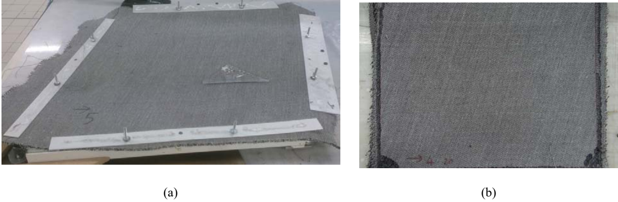
FIGURE 1. Commingled fabric (specified Tab. 1) (a) during the shearing step and (b) before consolidation at 20° shear angle with an ultrasonic welding line on the edges.
