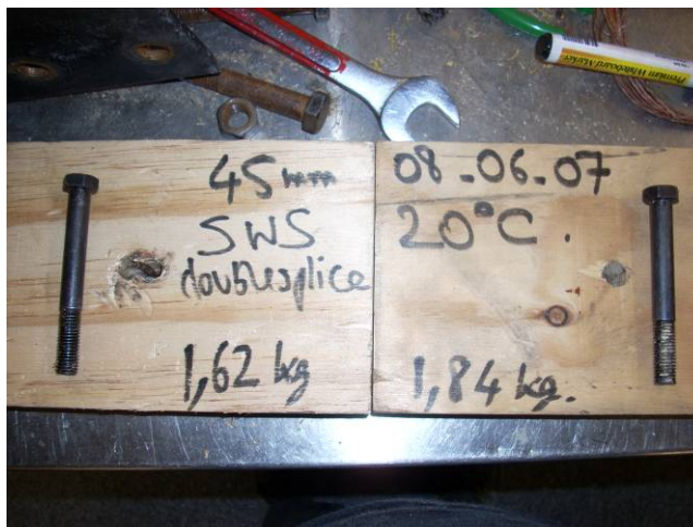
Ambient test on a sws connection with 45 mm timber and 12 mm steel plates on the sides. The bolts are straight so the failure is mode.
