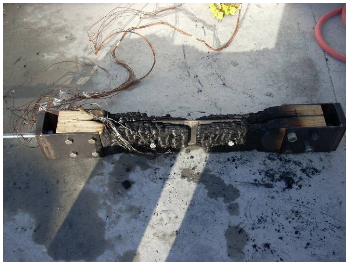
Wsw connection with one bolt after a fire test
