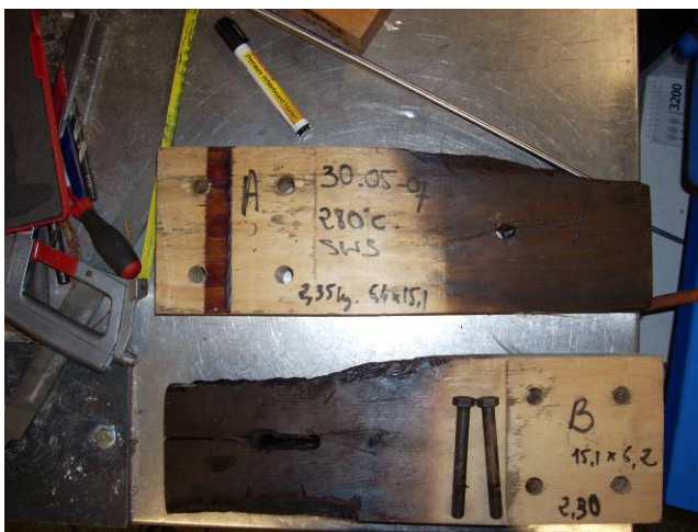
280 C heating test on a sws connection with 63 mm timber. The wood started charring on the sides. The bolts are straight so this is mode j.
