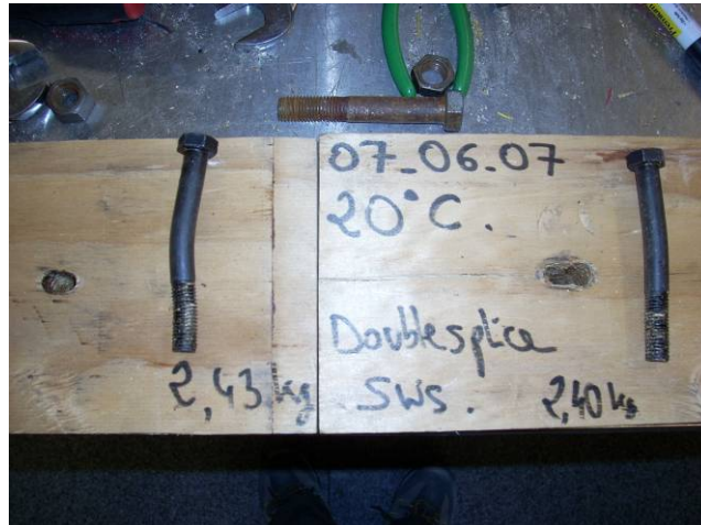
Ambient test on a sws connection with 63 mm timber and 12 mm steel plates on the sides. The bolts seems to be bent on mode m.
