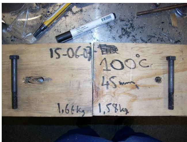
100 C heating test on a sws connection made of 45 mm timber. The bolts are straight so the mode of failure is mode j.
