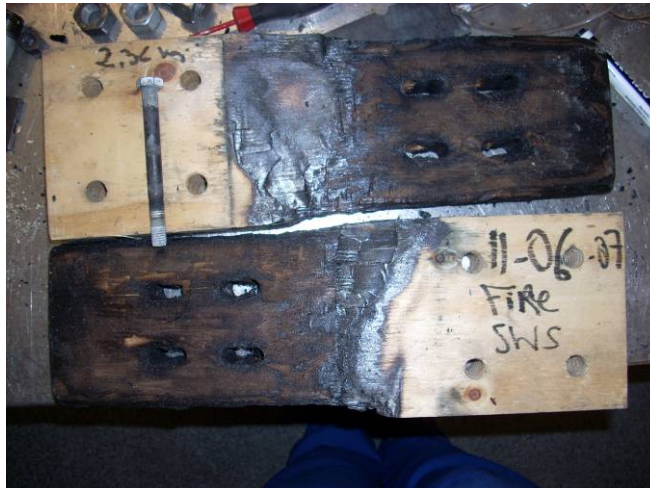
Sws connection with four bolts after a fire test once the char has been removed. The mode of failure is mode j (the timber is crushed)
